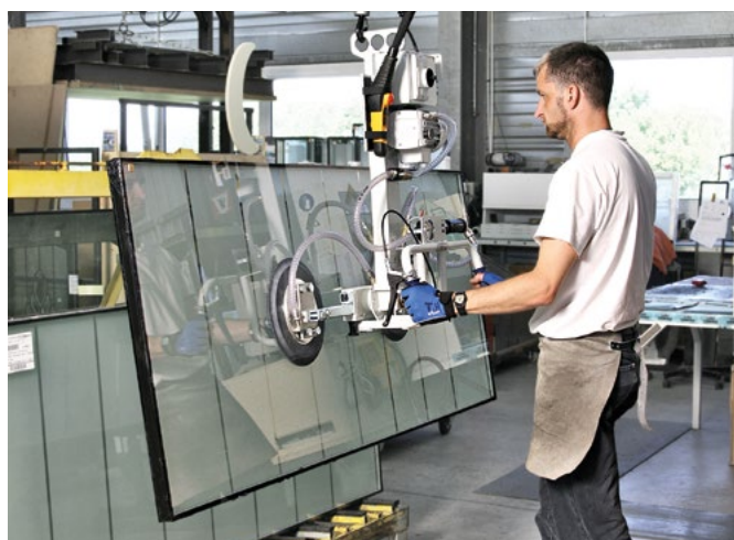
VacuMaster Window for vertical handling of glass elements
